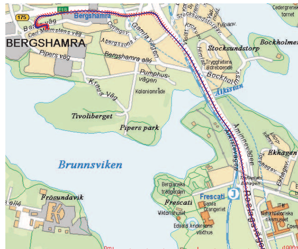
Figure 5.2: Estimated trajectory (blue solid line) and GPS-receiver position estimates (red crosses) from the field test. (Map: © 2006 Stockholms stadsbyggnadskontor)
