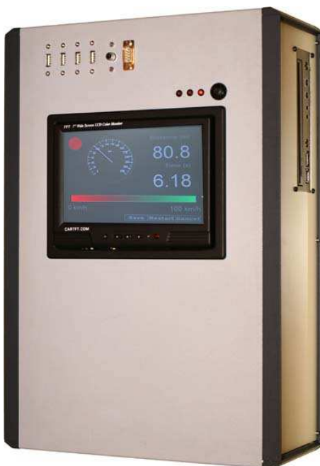
Figure 4.2: The TRÖGE testbed comprising an industrial PC, a touch-screen display, and several peripheral devices.
